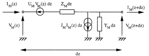
Fig. A.1. Per unit length model of the fundamental mode propagating in an inhomogeneous chiral anisotropic medium.
