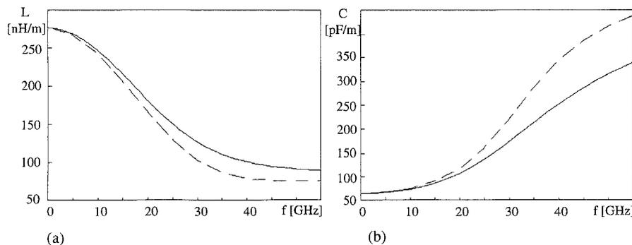
Fig. 8. Frequency-dependent transmission line parameters for the structure of figure 6 (——: anisotropic/---: isotropic): (a) inductance parameter  $L(\omega)$ , (b) capacitance parameter  $C(\omega)$ .
