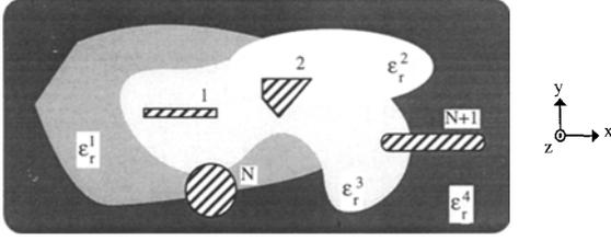
Fig. 1. General uniform waveguide structure with  $N + 1$  conductors.
