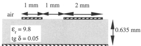
Fig. 2. Cross section of the asymmetric two-line microstrip configuration.
