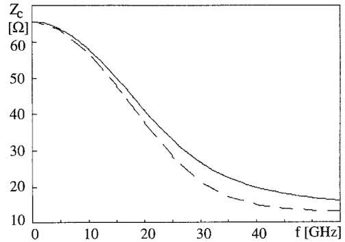
Fig. 9. Frequency-dependent characteristic impedance  $Z_c(\omega)$  for the structure of figure 6 (——: anisotropic/---: isotropic).
