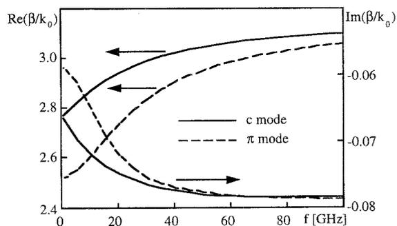
Fig. 3. Frequency-dependent propagation factors of the fundamental modes of the structure of figure 2.
