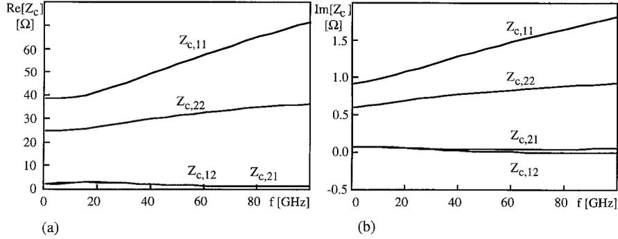
Fig. 5. Frequency-dependent elements of the characteristic impedance matrix  $Z_c(\omega)$  for the structure of figure 2.
