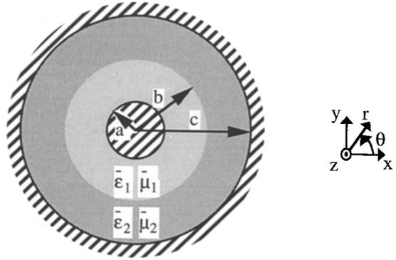
Fig. 6. Cross section of a coaxial cable filled with an inhomogeneous (an)isotropic dielectric.
