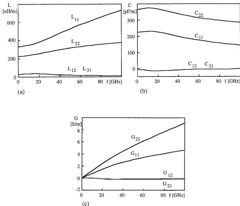
Fig. 4. Frequency-dependent transmission line parameter matrices for the structure of figure 2: (a) inductance matrix  $\mathbf{L}(\omega)$ ; (b) capacitance matrix  $\mathbf{C}(\omega)$ ; (c) conductance matrix  $\mathbf{G}(\omega)$ .
