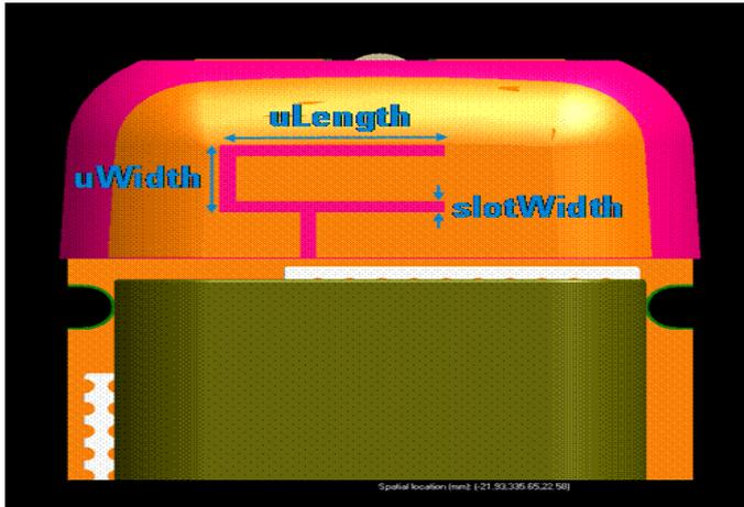
Figure 1: Non-Planar Inverted-F Antenna
