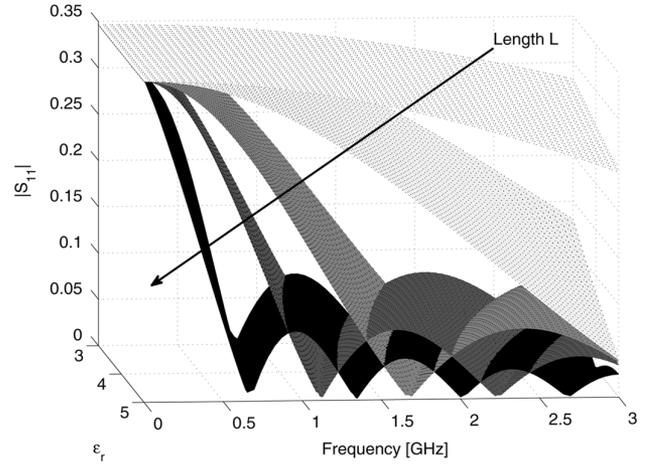
Fig. 3. Reflection coefficient  $S_{11}$  for  $L = 1, 2, 4, 6, 10$  cm.
