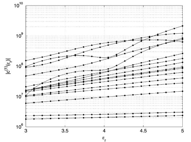
Fig. 5. Trajectories of all 1-D complex residues  $c_p^{(1)}(\epsilon_r)$  corresponding to all poles  $b^{(2)}$  of one 2-D complex residue  $c_p^{(2)}(\epsilon_r, L)$ : data evaluated in 20 values of  $\epsilon_r$  (dots), fit (solid line).
