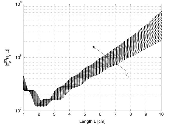
Fig. 4. Trajectories of one 2-D complex residue  $c_p^{(2)}(\epsilon_r, L)$  corresponding to pole  $a_p$ : data evaluated in 20 values of  $\epsilon_r$  and 50 values of  $L$  (dots), fit (solid line).
