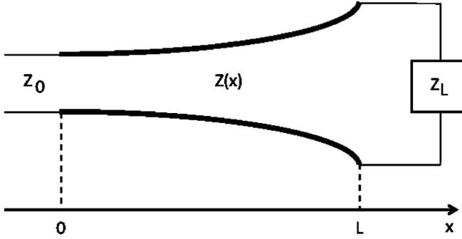
Fig. 1. Exponential tapered microstrip transmission line [10].
