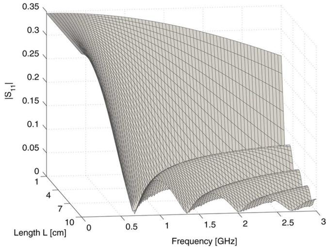
Fig. 2. Reflection coefficient  $S_{11}$  for  $\epsilon_r = 5$ .
