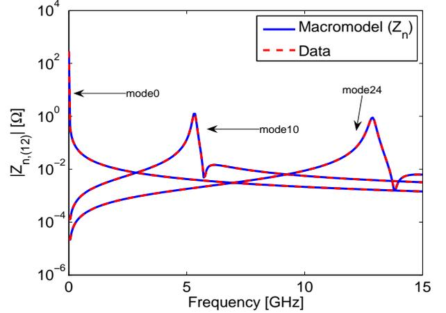
Figure 3: Magnitude of  $Z_{n,(12)}$  (modes  $n = \{0, 10, 24\}$ ,  $S = 295 \mu\text{m}$ ).
