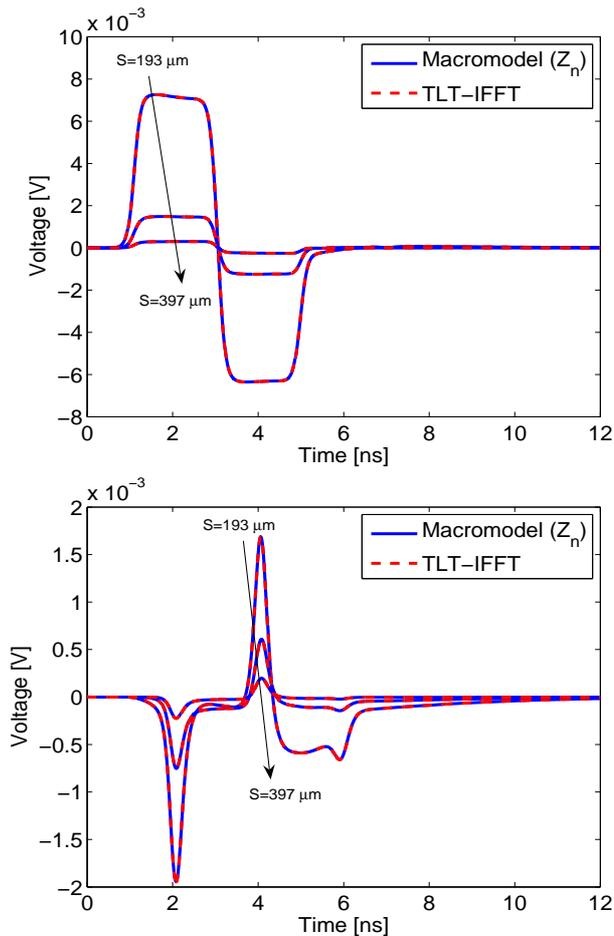
Figure 4: Input and output voltages of the victim line terminated on  $R_{NE} = 50 \Omega$  and  $R_{FE} = 50 \Omega$ ,  $C_{FE} = 1 \text{ pF}$  ( $S = \{193, 295, 397\} \mu\text{m}$ ).
