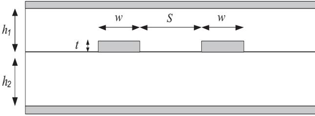
Figure 1: Cross section of the two coplanar striplines.
