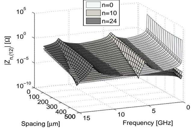
Figure 2: Magnitude of the parametric macromodel of modal impedance  $Z_{n,(12)}$  (modes  $n = \{0, 10, 24\}$ ).
