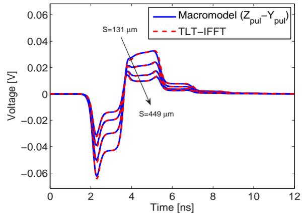
Fig. 10. Input and output voltages of the victim line terminated on  $R_{NE} = 50 \Omega$  and  $R_{FE} = 50 \Omega$ ,  $C_{FE} = 1 \text{ pF}$  ( $S = \{131, 233, 346, 449\} \mu\text{m}$ ).
