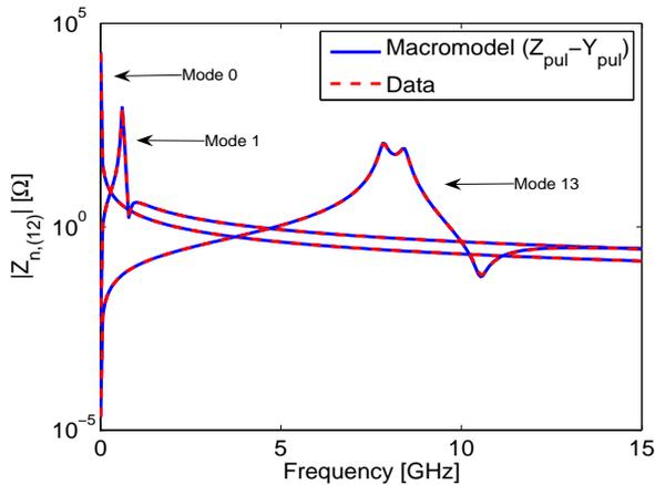
Fig. 3. Magnitude of  $Z_{n,(12)}$  (modes  $n = \{0, 1, 13\}$ ,  $S = 346 \mu\text{m}$ ).
