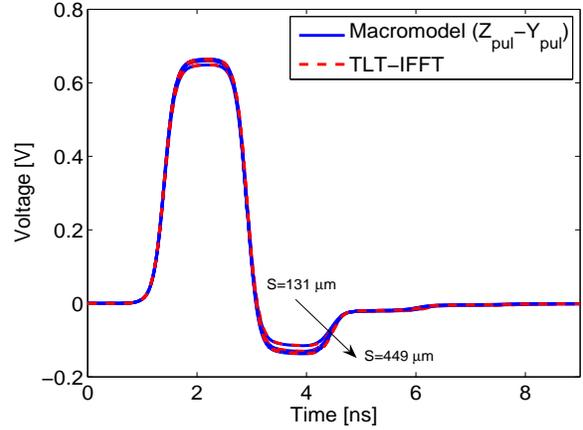
Fig. 9. Input voltage of the driven line terminated on  $R_S = 50 \Omega$  and  $R_L = 50 \Omega$ ,  $C_L = 1 \text{ pF}$  ( $S = \{131, 233, 346, 449\} \mu\text{m}$ ).
