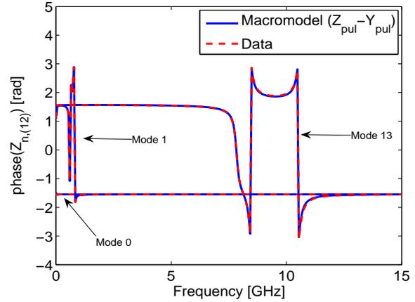
Fig. 4. Phase of  $Z_{n,(12)}$  (modes  $n = \{0, 1, 13\}$ ,  $S = 346 \mu\text{m}$ ).
