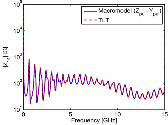
Fig. 6. Magnitude of  $Z_{14}$  ( $S = 131 \mu\text{m}$ ).
