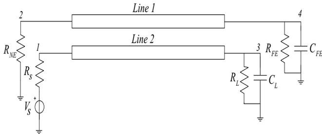
Fig. 8. Two coupled microstrips with linear terminations.
