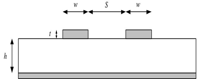
Fig. 1. Cross section of the two coupled microstrips.
