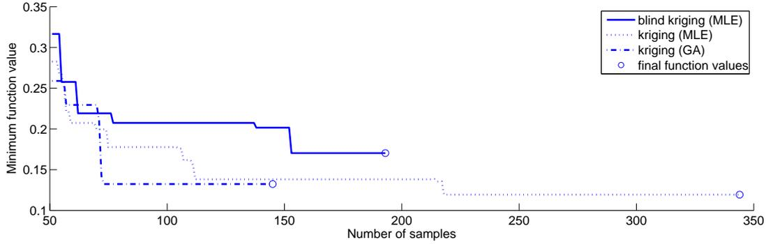
Figure 4: Evolution of the minimum function value versus the number of samples evaluated
