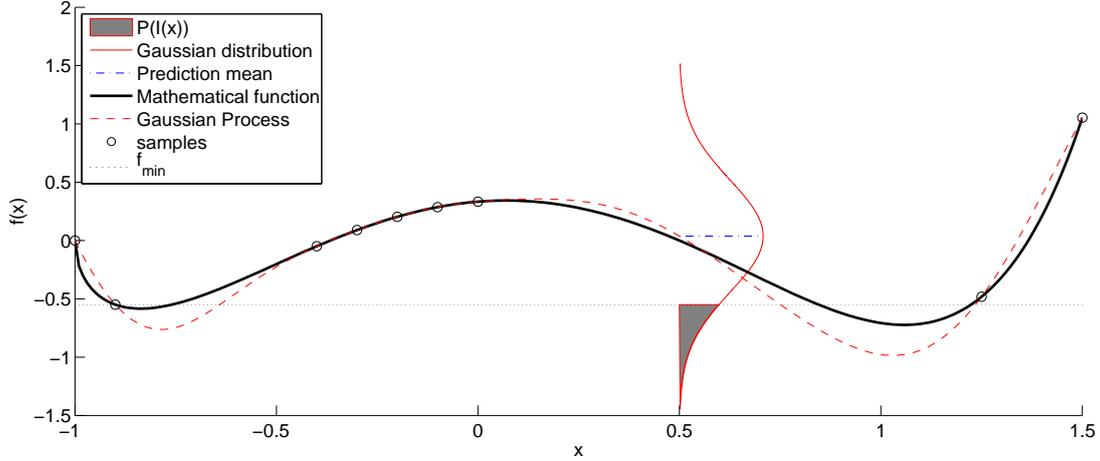
Figure 2: Graphical illustration of Gaussian Processes and  $E[I(x)]$
