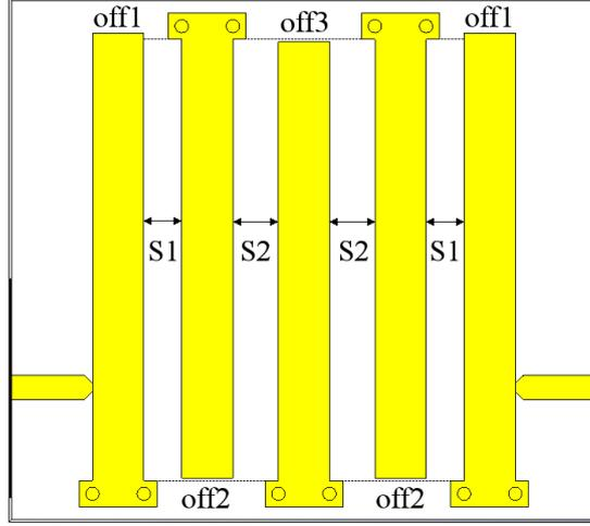
Figure 3: Layout view of the 3D narrow-band filter
