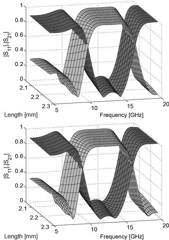
Fig. 2. Magnitude of the trivariate models of  $S_{11}$  (light grey surface) and  $S_{21}$  (dark grey surface) for  $S = 0.091$  mm (top) and  $S = 0.171$  mm (bottom).
