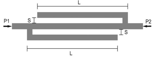
Fig. 1. Geometry of the double folded stub microstrip bandstop filter [15].
