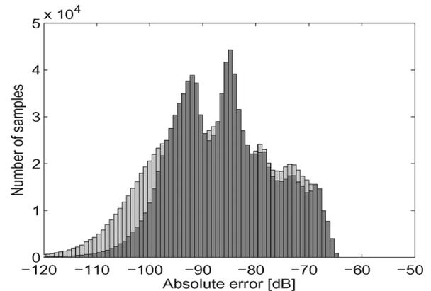
Fig. 3. Histogram: error distributions of the trivariate models of  $S_{11}$  (light grey) and  $S_{21}$  (dark grey) over 1080000 validation samples.
